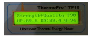
Once properly mounted, the TP10's programming menu guides the installer through the final steps to optimize transducer placements, displaying advanced signal diagnostics that confirm correct sensor orientation. For this reason, ultrasonic transducers are always installed when the pipe is fully charged (flow, however, is not necessary) to provide an accurate acoustic profile. These diagnostic values are then continuously monitored and may be viewed
